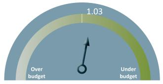
The cost performance index (CPI) is the measure of the efficiency of expenses spent. CPI is equal to budgeted cost divided by actual cost. A value higher than one indicates a favorable condition, while a value less than one would be considered unfavorable.
